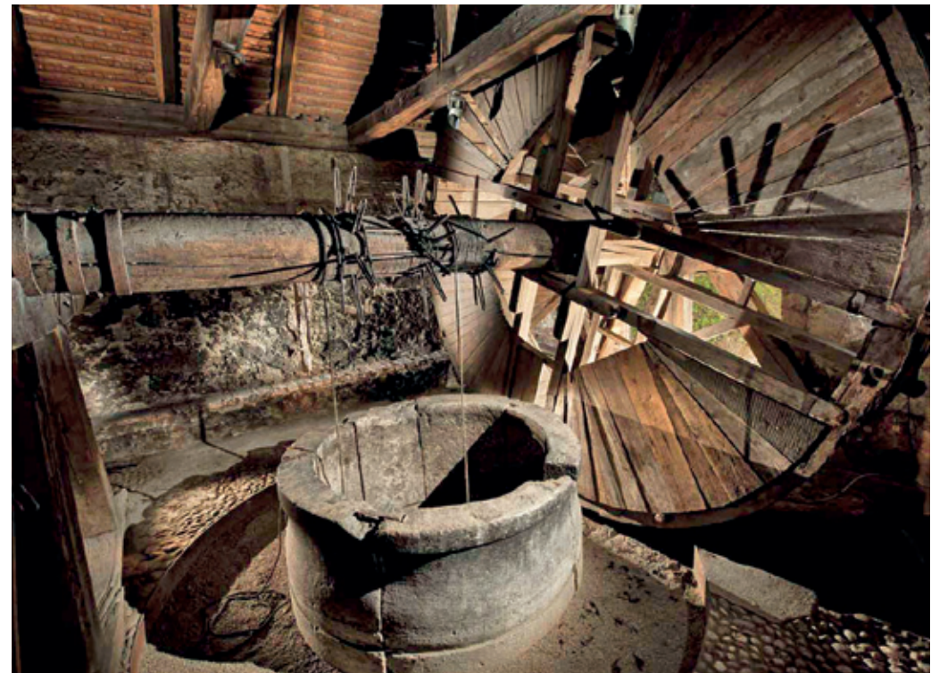
Notranjost vodnjaka s pohodnim gonilnim kolesom pred Ljubljanskim gradom/The interior of the well with a walking drive wheel in front of the Ljubljana Castle (foto/photo: Branko Čeak)
